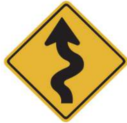
Winding road left ahead
